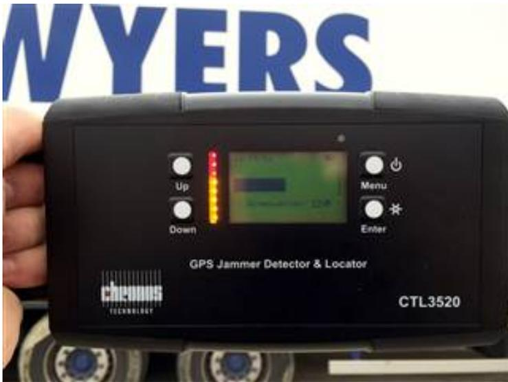
A device used by authorities to detect truckers using jammers. Chronos Technology Ltd.
